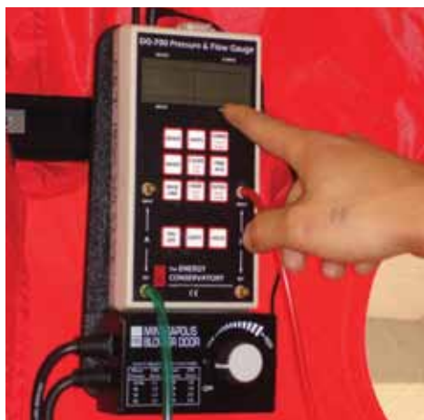
Taking measurements during the leak-revealing blower door test.
